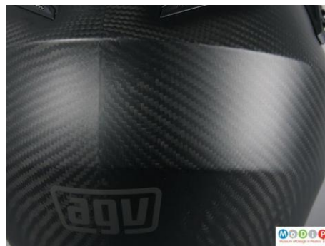
Close-up of carbon fibre sheet
